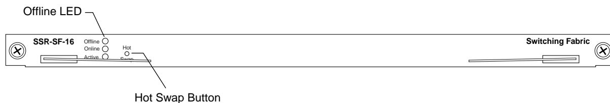
Figure 4. Location of Offline LED and Hot Swap Button on a Switching Fabric Module
